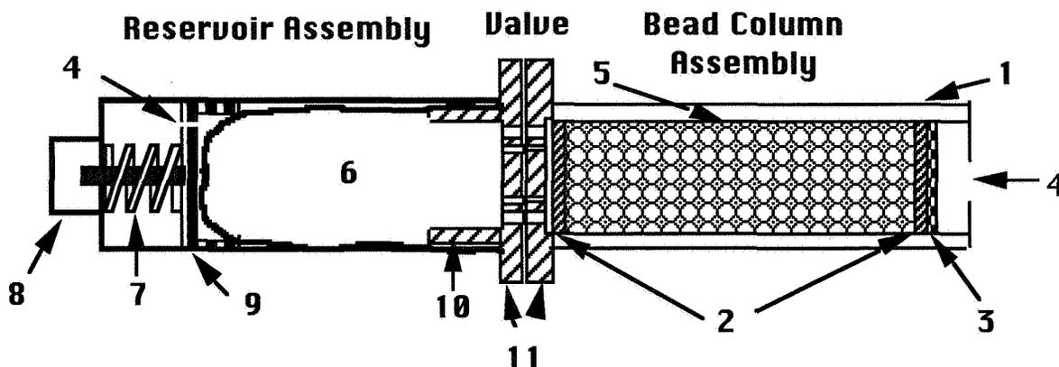
Fig. 1. Conceptual schematics of the modified capillary test bed assembly (CTB-M) used in the experiments conducted during the STS-63 mission.
