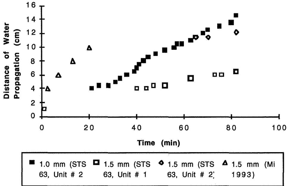
Fig. 3. Comparison of the capillary water propagation in experiments conducted in microgravity during the STS-63 mission and an experiment conducted on the MIR Space Station (Yendler, et al., 1994).
