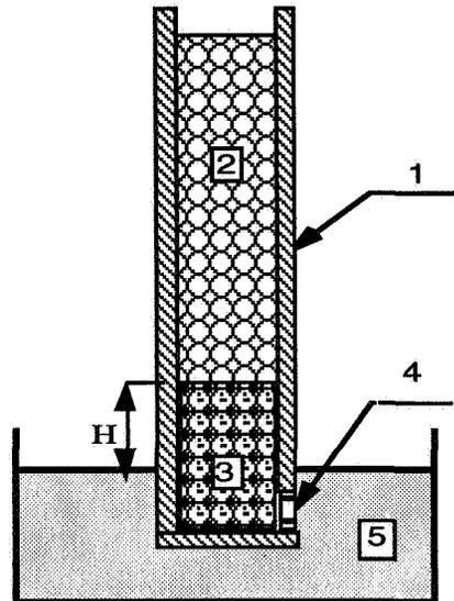
Fig. 4. Conceptual diagram of an apparatus to determine the amount of capillary rise,  $H$ , in a bed of glass beads.
