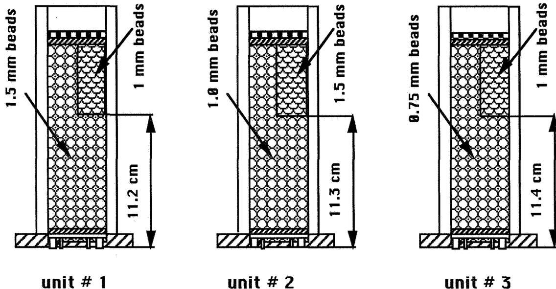
Fig. 2. Diagrammatic representation of the matrix composition of the CTB-M units for the microgravity experiments conducted during the STS-63 mission.
