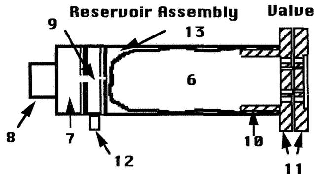
Fig. 5. Conceptual diagram of a modified CTB-M reservoir assembly (only components of the reservoir assembly are shown, see Fig. 1).
